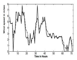
Figure 4. ONTARIO actual wind speed (solid line) and predicted wind speed using passive aggregation model (dotted line) for three days testing data
