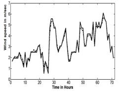
Figure 3. QUEBEC actual wind speed (solid line) and predicted wind speed using passive aggregation (dotted line) for three days testing data
