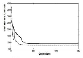
Figure 5. Quebec Best fitness functions of wind speed prediction using both the standard model (solid line) and the passive aggregation model (dotted line).
