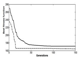
Figure 6. ONTARIO Best fitness functions of wind speed prediction using both the standard model (solid line) and the passive aggregation model (dotted line).
