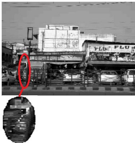
Figure 8. The estimated background obtained by block wise 4 bit requantization algorithm on 600 frames using 2 \times 2 blocks.
