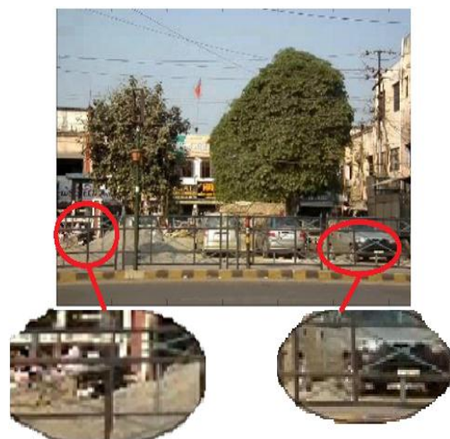
Figure 12. The estimated background using the with 4 bit requantized color algorithm on 600 frames.
