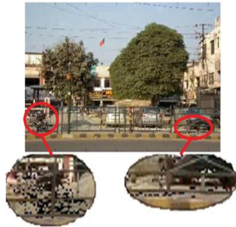
Figure 11. The estimated background in color using the color algorithm with 4 bit re-quantized images and 200 frames. The enlarged regions shows the pixels where no common frames are found across 3 channels of R, G, B.
