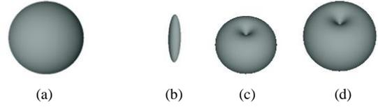
Figure 4. (a)  $d(X)=1$ : a sphere. (b)  $d_E(X)=1$ : an ellipsoid. (c) Erosion of the sphere in (a) by the ellipsoid in (b). (d) Partial erosion of the object in (c), which has a similar size with the sphere in (a).
