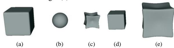
Figure 6. (a)  $d(X)=1$ : a cube. (b)  $d_{E1}(X)=1$ : a sphere. (c) Concave cube, obtained from the erosion of the cube in (a) by the sphere in (b). (d)  $d_{D2}(X)=1$ : restoring function of a cube. (e) Partial erosion of the concave object in (c) by using the cube in (d) as a restoring function.
