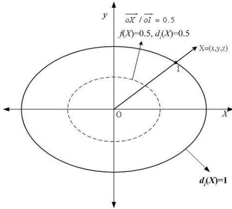
Figure 1. Influential region  $d_i(X) = 1$ , solid line, and the shape of soft object  $f_i(X) = (P \circ d_i)(X) = 0.5$ , i.e.  $d_i(X) = 0.5$ , dotted line.
