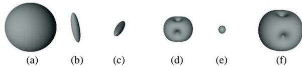
Figure 9. (a)  $d(X)=1$ : a sphere. (b)-(c)  $d_{E1}(X)=1$  and  $d_{E3}(X)=1$ : ellipsoids. (d) Sphere with four holes, obtained from the erosion of the sphere in (a) by the ellipsoids in (b)-(c). (e)  $d_{D2}(X)=1$  and  $d_{D4}(X)=1$ : restoring functions of a sphere. (f) Double partial erosion of the object in (d) using the sphere in (e) as restoring functions.
