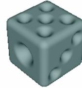
Figure 2. A die generated from a difference operation of a cube from 21 spheres.
