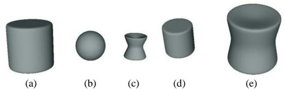
Figure 7. (a)  $d(X)=1$ : a cylinder. (b)  $d_{E1}(X)=1$ : a sphere. (c) Concave cylinder, obtained from the erosion of the cylinder in (a) by the sphere in (b). (d)  $d_{D2}(X)=1$ : a restoring function of a cylinder. (e) Partial erosion of the concave object in (c) using the cylinder in (d) as a restoring function.
