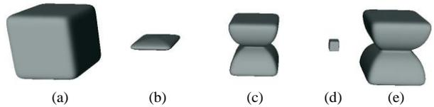
Figure 11. (a)  $d(X)=1$ : a cube. (b)  $d_{E1}(X)=1$ : a cubic disk. (c) Erosion of the cube in (a) by the disk in (b). (d)  $d_{D2}(X)=1$ : a restoring function of a cube. (e) Partial erosion of the object in (c) using the cube in (d) as a restoring function.
