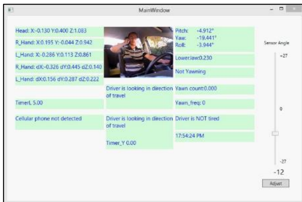
Figure 15. Driver with cellular telephone in hand-no warning.
