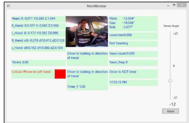
Figure 16. Driver with cellular telephone in hand 1-warning displayed.
