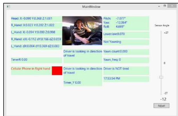
Figure 17. Driver with cellular telephone in hand 2-warning displayed.
