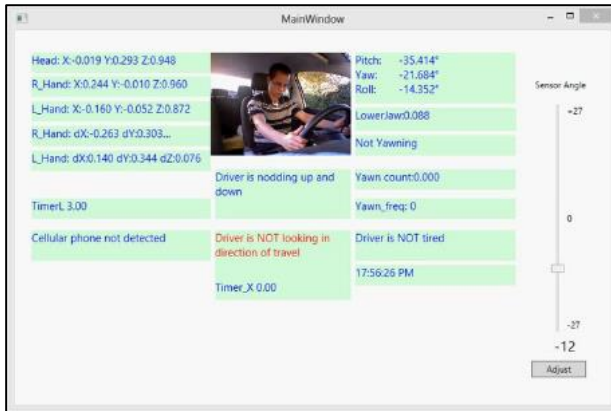
Figure 19. Head pose warning message-driver looking down.
