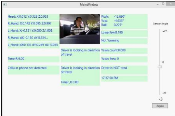
Figure 14. Driver not yawning with head facing direction of travel.
