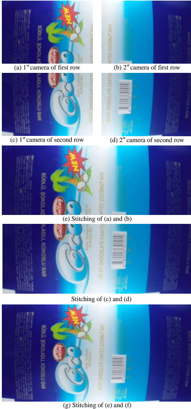
Figure 6. An example of 2x2 camera array.
