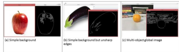
Figure 4. Defected results of edge detection using traditional method directly.
