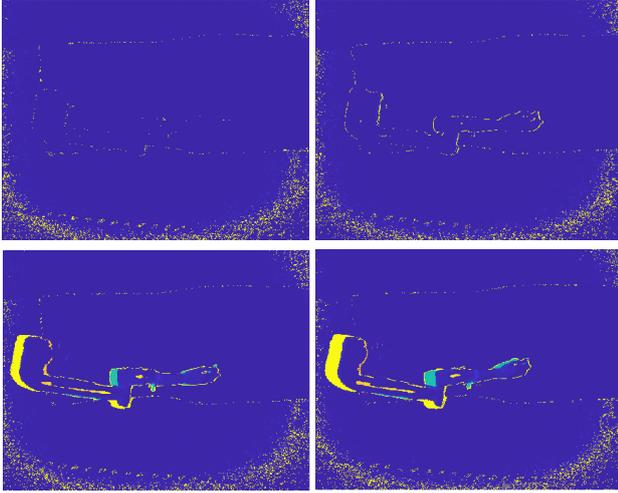
Figure 2. Depth difference image for each of the recorded movement categories, i.e. rest (top left), random light motion (top right), random strong motion (bottom left) and seizure-like motion (bottom right).
