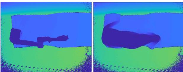
Figure 1. Depth images of hand phantom mounted onto the robotic arm for data acquisition without (left) and with (right) duvet as seen from and recorded by the Kinect v2 camera.
