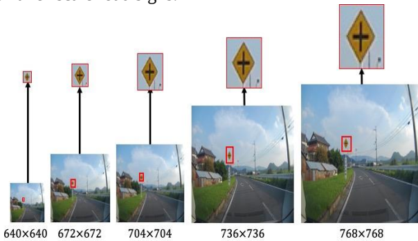
Figure 10. Training with multi-scale inputs
