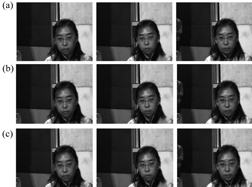
Fig. 8. Experimental output images of the preprocessing techniques on the dataset SMIC. (a) Input micro expression frames. (b) Images after illumination control by EPHF technique. (c) Images obtained on the output of YOLOv3.
