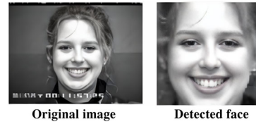
Fig. 1. Face detection with the Viola and Jones algorithm [13].
