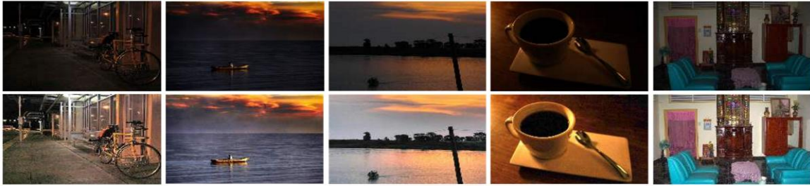
Fig. 8. The outcomes of applying the proposed RISSR algorithm on low light images from ExDark dataset (Batch 5). The first row are the degraded images, the second row are the enhanced images using \alpha = 0.51, 0.72, 0.91, 0.59, 0.87 , respectively.
