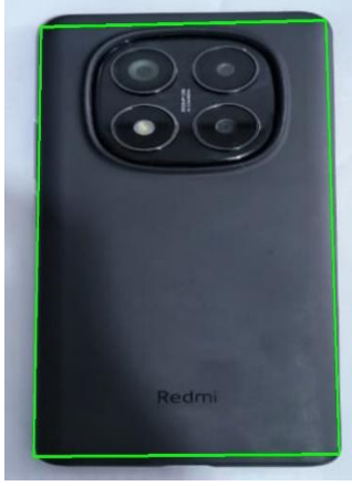
Fig. 5. Contour detection of item placement inside the enclosure box.
