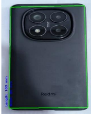
Fig. 7. Object contour with length and width in millimeters.
