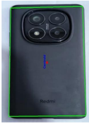
Fig. 6. External contour with marked centroid.
