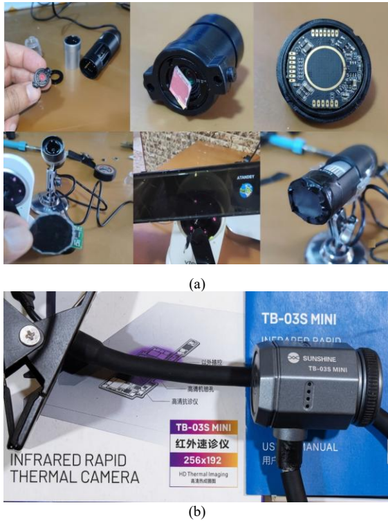
Fig. 3. Proposed system components and reference camera. (a) Making infrared thermal imaging (IR), (b) Reference thermal camera (SUNSHINE TB-03SMINI).
