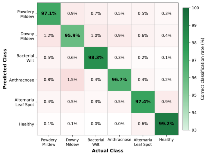
Fig. 4. Normalized confusion matrix—PSO-SVM classifier (values represent % of actual class samples correctly/incorrectly classified).
