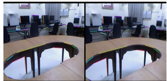
Figure 7. Shows indoor scenario of lab where the colorful lines shown are the detected lines in 3D. The matched lines in the two frames are shown by same color.
