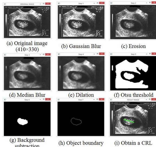
Figure 4. Image processing of CRL estimation
