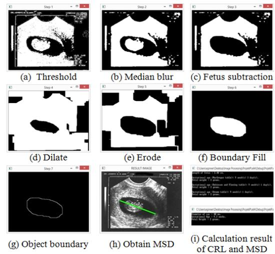
Figure 5. Image processing of automatic MSD estimation
