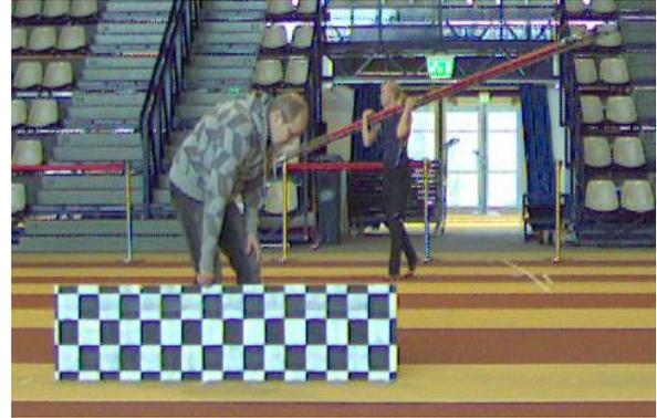
Figure 3. Calibration chessboard at the projection plane
