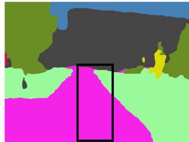
Figure 3. A segmented image obtained from a side camera just before a robot entering to intersection.
