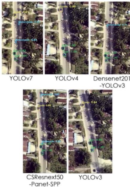
Figure 16. Approximately identical image comparison of detected objects for each model.
