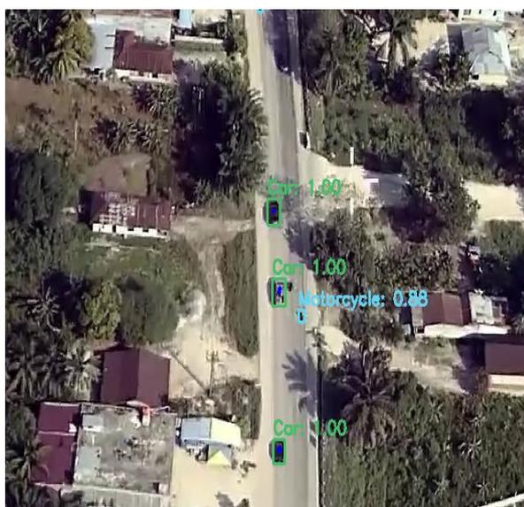
Figure 3. MAP results from object class detection from UAV datasets on public highways using CSResNext50-Panet-SPP.
