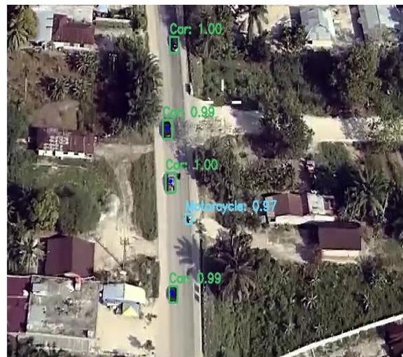
Figure 2. MAP results from object class detection from UAV datasets on public highways using DenseNet201-YOLOv3.
